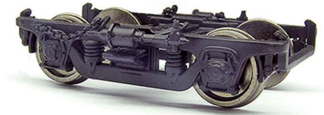
Rapido Trains (Discontinued) //41-ER? The Rapido model was included in their Osgood Bradley "American Flyer" cars and included both solid and roller bearing versions as appropriate.
